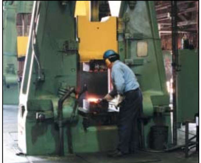
One of the many hammers capable of producing forgings up to 50 lbs.
