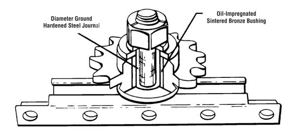
Chain Tightener (Less Idler Sprocket) No. E-5006
