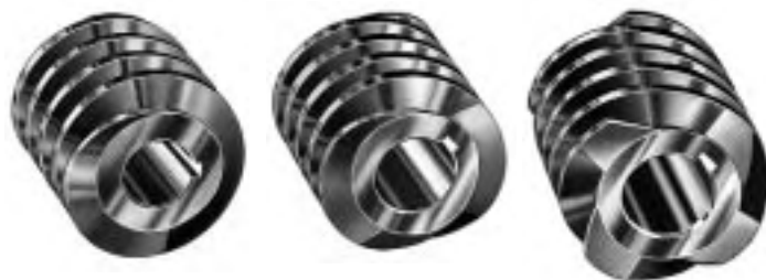
Single, Double, quadruple thread worms.
