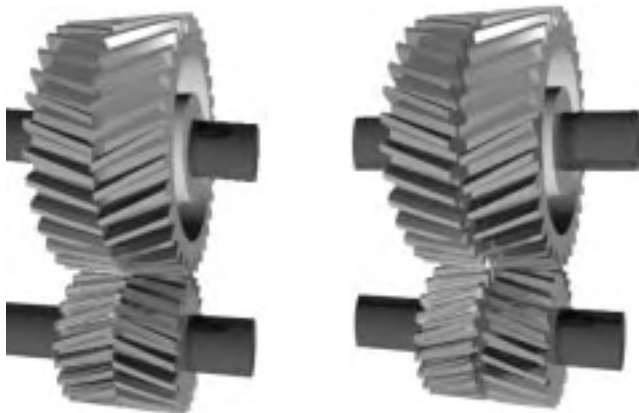
Herringbone gears have opposed teeth joined in middle.
