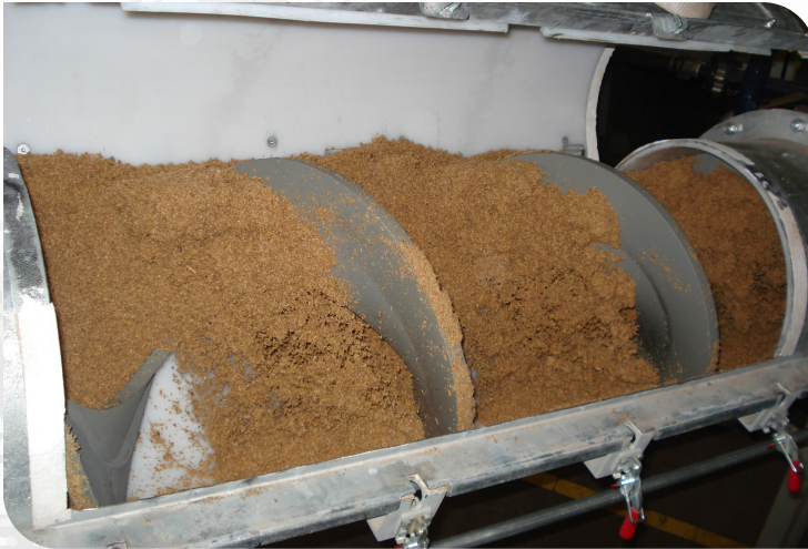
Shaftless Screw with UHMW Liner Conveying Sticky Humid Beer Brewing Grains
